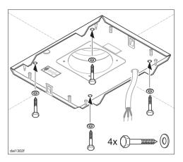
■ Screw the mounting plate through the ceiling and into the structural framing using 8 x 60 lag bolts and washers. Once tight, make sure that the mounting plate can safely support the weight of the hood.
